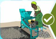
Use appropriate shelling methods such as motorised shellers to avoid breakage
